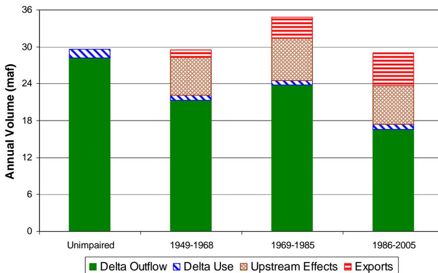
**Figure 6. Comparison of annual water use during the three study periods (maf/year) compared to the Unimpaired flows from 1921-2003. Unimpaired data from DWR (2006) and other from Dayflow web site (Neglects upstream groundwater withdrawals).**
