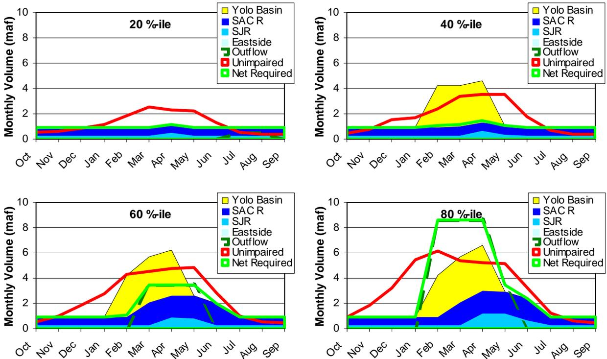
Figure 10. Preliminary monthly flow recommendations and unimpaired flows for different percentile years (top – 20<sup>th</sup> & 40<sup>th</sup> %-ile) and (bottom – 60<sup>th</sup> & 80<sup>th</sup> %-ile). Dark, medium and light blue represent Sacramento, San Joaquin and Eastside inflows. The dashed dark green line represents the prescribed outflow levels while the light green solid line is the net required flows by the maximum of the inflow or outflow. The red line is unimpaired flow.
