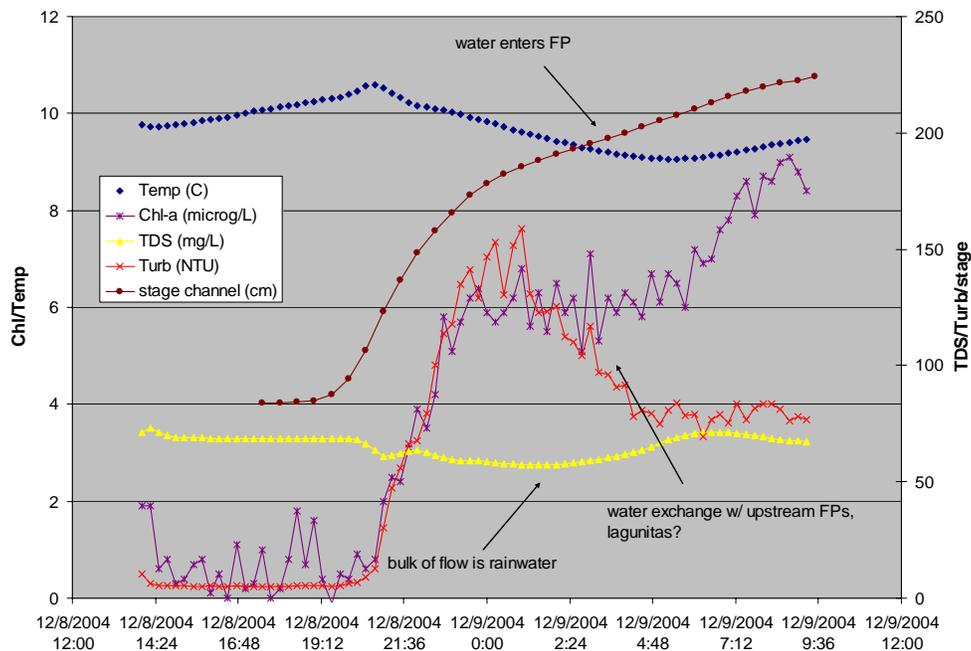
**Figure 4.** This graph displays data collected from the YSI sonde installed at the Corps breach.
