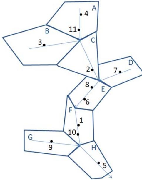
Figure 2 – Example watershed. Sub-basins are outlined and labeled A-H. Users are represented by black dots and labeled 1-11. Arrows indicate direction of flow.
