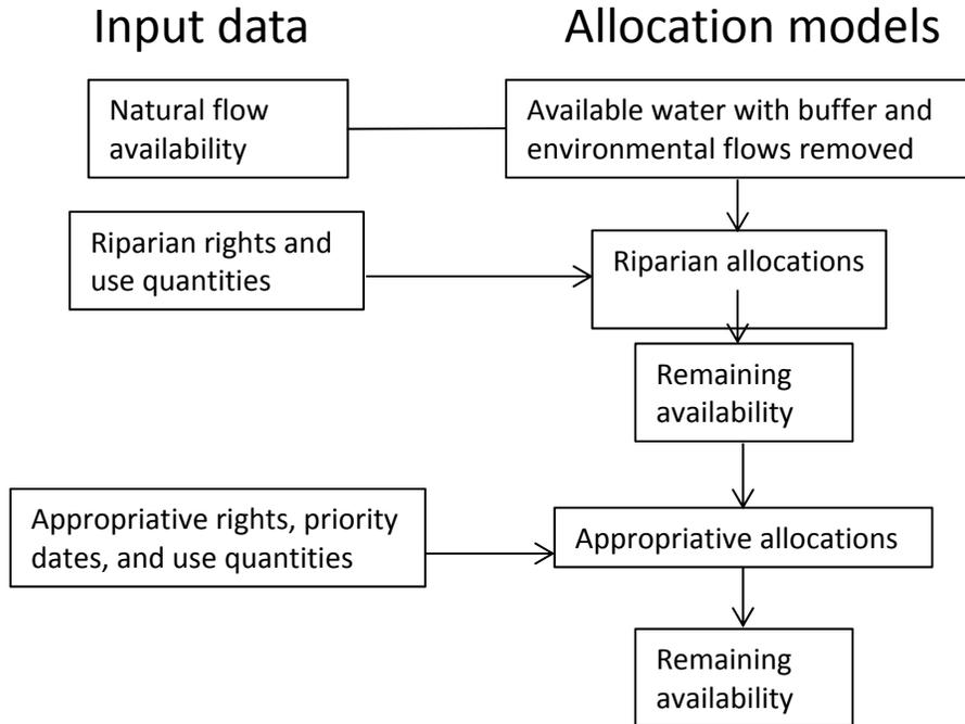
Figure 1 – DWRAT data flow. Boxes on left indicate required input data. Boxes on right indicate phases of allocation and reductions in availability.
