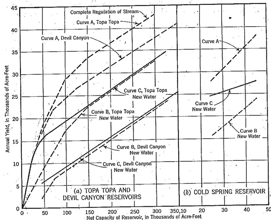
FIG. 6.—CAPACITY-YIELD CURVES FOR SURFACE RESERVOIRS
