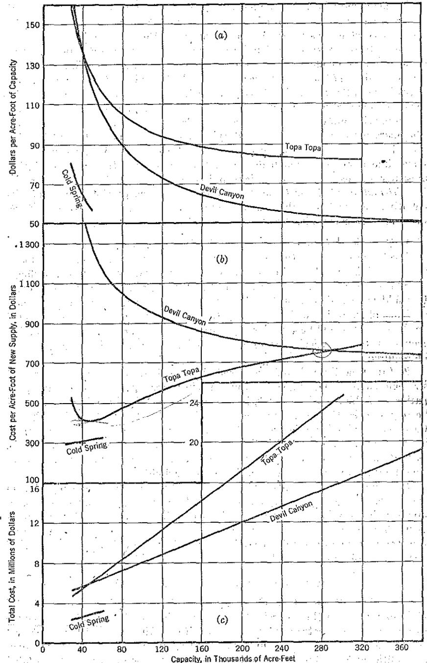
FIG. 7.—COST OF SURFACE RESERVOIRS (1950)
