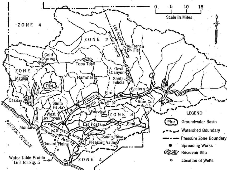
FIG. 1.—GROUND-WATER BASINS IN VENTURA COUNTY, CALIFORNIA
