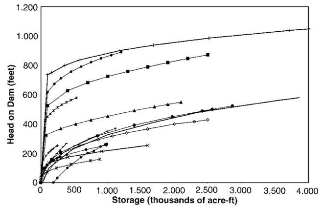
**Fig. 3.** Head-storage curves for same 16 large reservoirs in California
