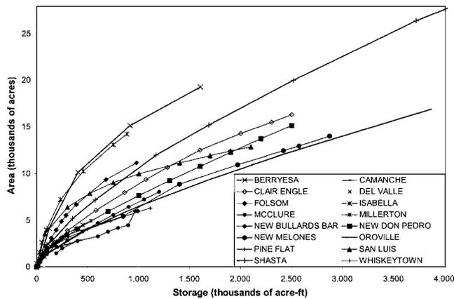
**Fig. 2.** Area-storage curves for 16 large reservoirs in California
