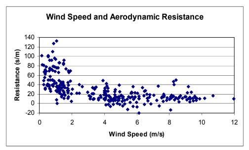
Figure 3. Relationship of wind speed (m/s) to measured resistance (s/m).
