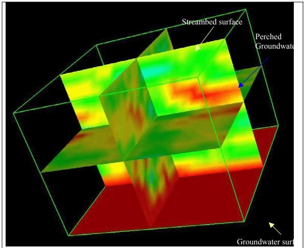
**Figure1**: Contour plot of sediment water content at the Cosumnes River three months after flow ceased. Red color represents saturated sediments and blue being dry. The horizontal plane spans 100 m in both directions and the vertical distance is 15 m, showing a 5:1 vertical exaggeration.
